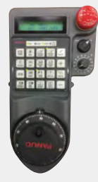
Manual operation panel
